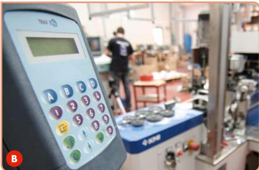
*For the production the wiring department has got automatic machines. The processing includes the cutting, the stripping of the cable, the crimping of the terminals and the insertion of the isolation sleeves. Gbm only uses marked unipolar cable: Silicone IMQ, H05S-K, PVC HT°90 H05V2-K, Fiberglas braid silicone IMQ H05SJ-K, etc. and terminals of various materials: brass, tinned brass, steel, silver nichel and others in accordance with DIN regulation of major manufactures.*
